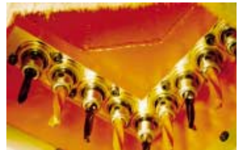
The 9 spindle vertical drill is ideal for line hole drilling and individual point-to-point drilling for various applications. The Drill Head has FULL TABLE COVERAGE
